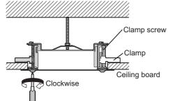
6. Secure the bracket by attaching and tightening a nut (not included) to the anchor bolt.
